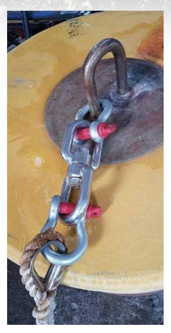
▲ The correct method of attachment to a mooring buoy: buoy ring - shackle - swivel - shackle to the mooring lines, with a metal thimble to prevent wear and tear on a particular spot. This allows movement of all of the components in the mooring system, which absorbs excess energy.
