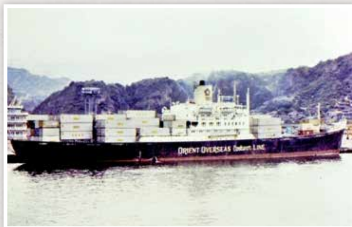
Hongkong Success 1972 – a 1st generation boxship converted from an old break-bulk general cargo ship
