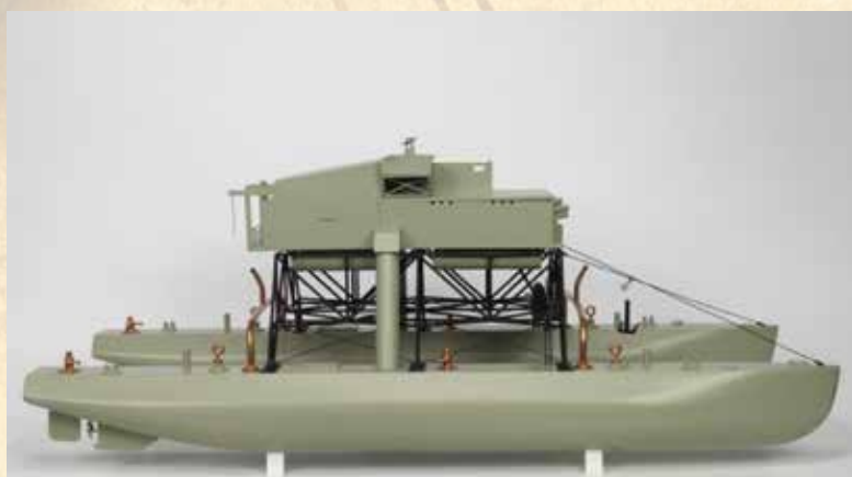
The model of the LCG(T) that was tested in a tank, now in the Imperial War Museum
