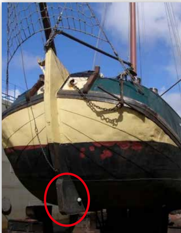
Figure 2: Loefbijter on a Dutch sailing tjalk
